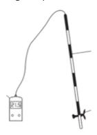
• Pebbleometer: A very basic device for measuring the size and shape of material found on a beach or in a river.
